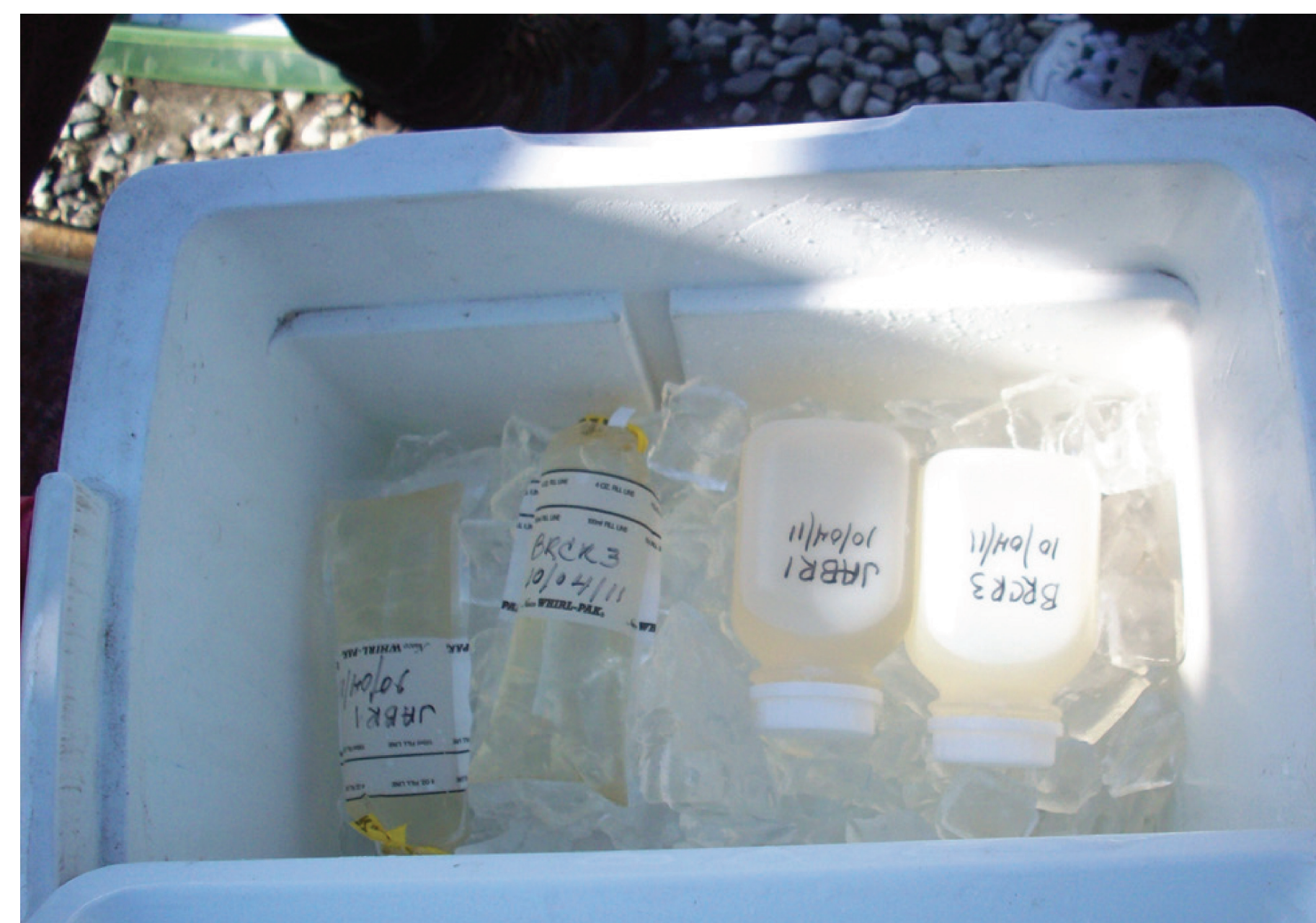
Labeled water samples are placed in a cooler with ice to preserve the integrity of the sample.
