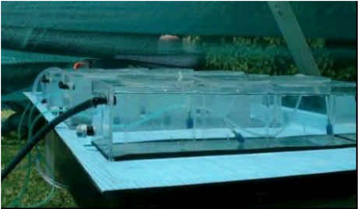
Plate 1: Overview of experimental setup, showing the four temperature regulated tanks with three chambers per tank.
