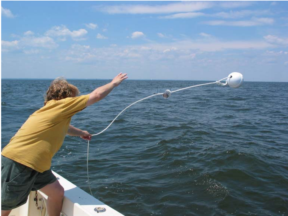
Plate 4. Deploying the incubation rig with buoy, perforated macroalgal chamber, sinker and bricks
