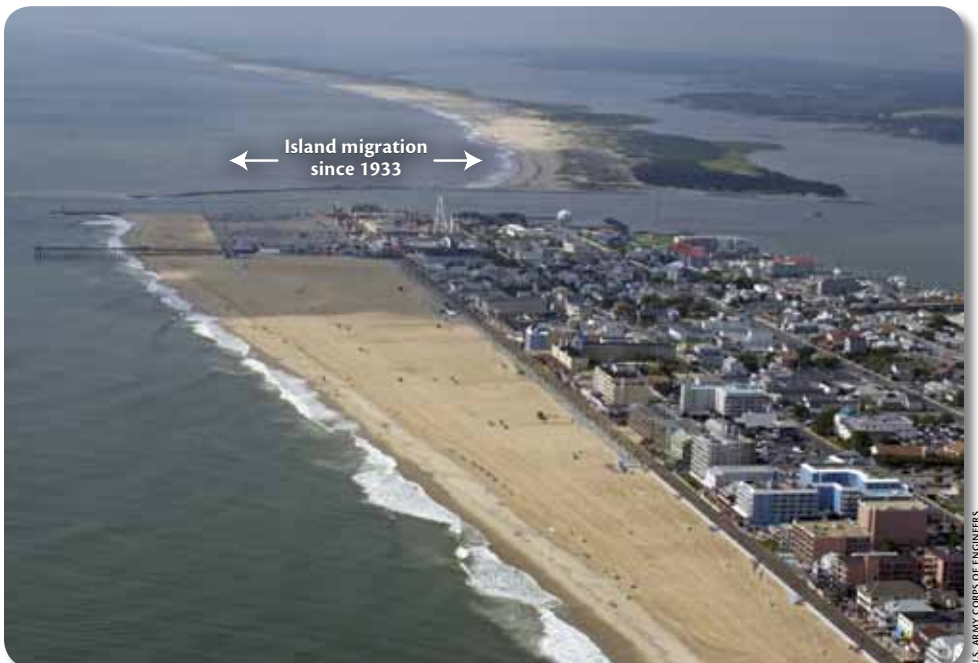
This aerial photo of Fenwick Island and Ocean City (foreground) and Assateague Island (background) shows how far the north end of Assateague Island has migrated landwards since the opening of the Ocean City Inlet in 1933.
