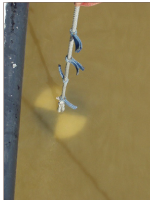
A Secchi disc is lowered into water to measure water clarity.
