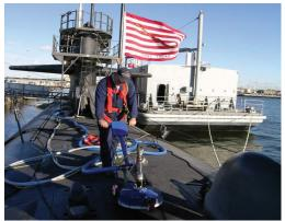
A sailor at Naval Station Norfolk, Virginia using a High Pressure Water Jet Blasting System to remove faulty non-skid deck surface. Previously, this was done by grinding. The new method reduces heavy metal-containing dust emmisions by 90%.
