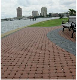
Pervious pavers installed at Naval Medical Center Portsmouth, Virginia help to reduce the area of impervious surface on the compound.
