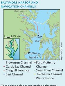
These channels are maintained through periodic dredging, with the material removed being placed in specified dredged material placement sites. Department of Defense
