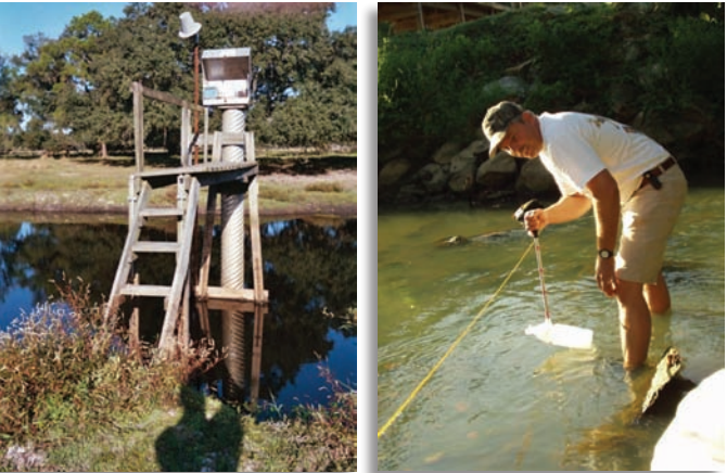
Water quality is collected by automatic data logger platforms and researchers throughout the Chesapeake Bay watershed. Water samples are taken back to the lab for nitrogen analysis.
