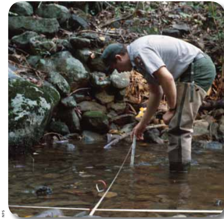
In order to monitor stream health, park staff take water quality measurements that include sediment, nutrients, pH, and water temperature.
