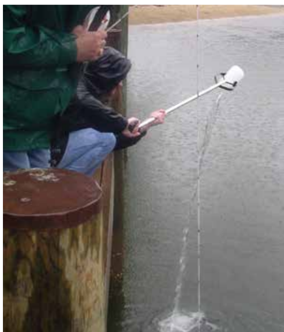
Figure 6.3. If sampling from a pier, use an extendable grab pole to hold the bottle under the surface. Make sure to rinse the bottle three time before collecting the sample.
