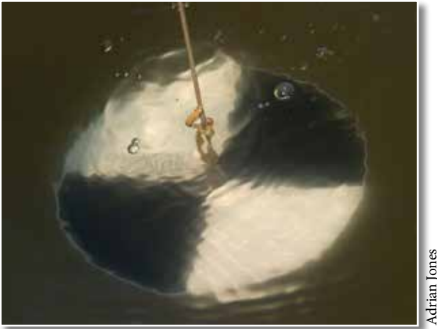
Figure 7.3. A Secchi disk being lowered into the water to measure water clarity.
