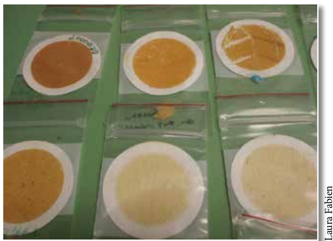
Figure 6.4. Filters with chlorophyll residue on them. The different colors represent the different amounts of chlorophyll in the water sample.
