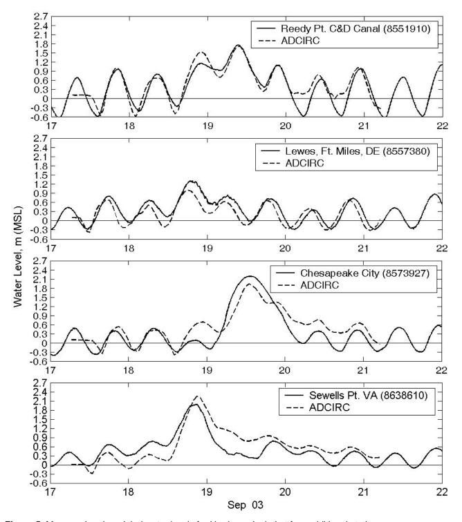
Figure 5. Measured and modeled water levels for Hurricane Isabel at four additional stations.
