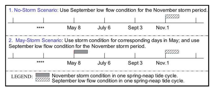
Figure 2. Example of the method used to simulate the Hurricane Juan event in May.
