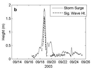
**Figure 3.** Panel a: comparison of predicted tidal elevation and observed water level at Gloucester Point from NOAA's destroyed tide gauge and the ADCP pressure record. Panel b: storm surge above astronomical tides and significant wave height (Hs) at Gloucester Point.
