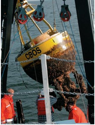
Figure 10. Damage to CBOS mid-Bay buoy after Isabel.
