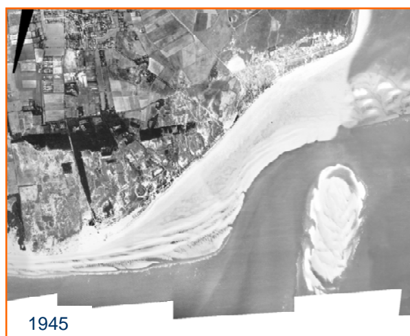
Figure 5. Human alteration of coastal processes. Dredging of the River Mersey, UK and the construction of training walls have altered sediment movement leading to erosion/accretion zones and closure of a channel in the area south west of Formby known as Taylors spit and the Formby channel between 1945 and 2002.
