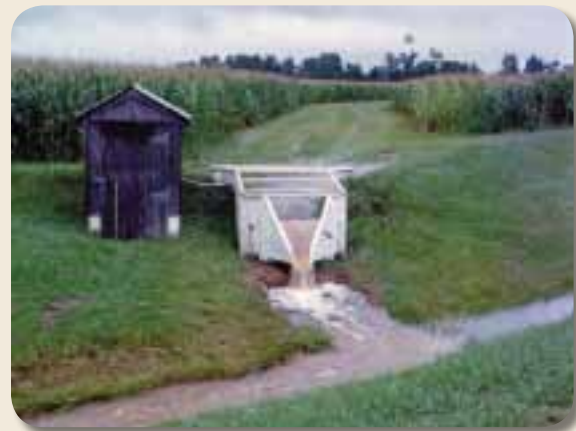
Surface runoff following a summer thunder storm flowing through a monitoring flume.
