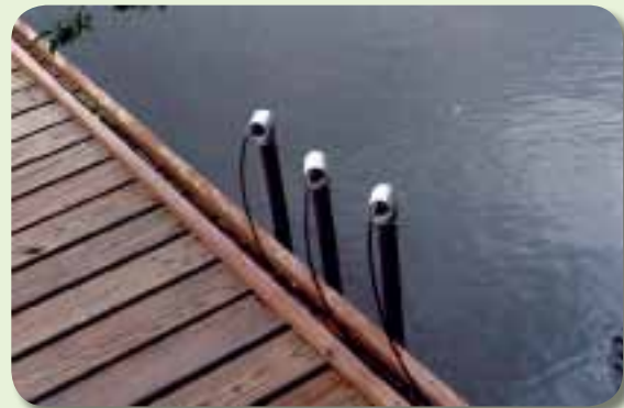
Wells equipped with pressure transducers for measuring hydraulic gradients in the intertidal groundwater discharge zone in the Wye River.
