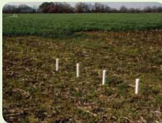
Well nest for monitoring shallow groundwater at different depths in a crop field.
