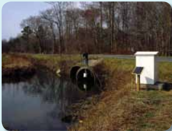
Automated stage recording device used to calculate stream discharge.
