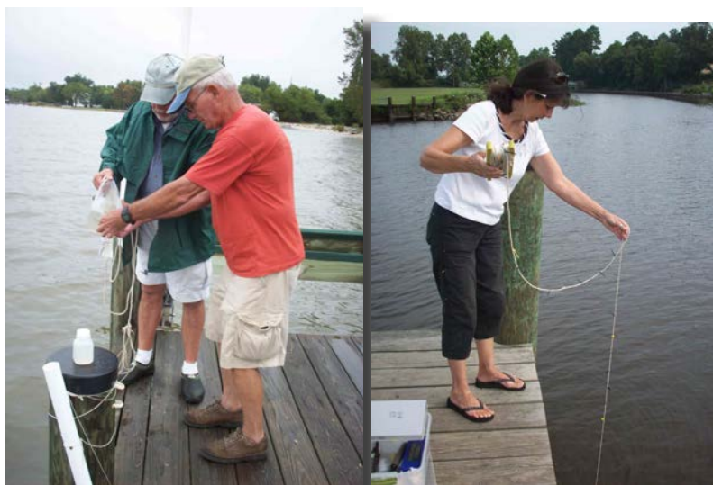
Figures 6-7: On left, Cyrus Marter and Ron Maher (l-r) acquire a nutrient sample on the Lower Nanticoke. On right, Susan Good measures the Secchi depth on the Marshyhope Creek.
