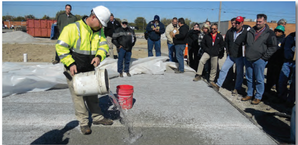
A demonstration shows the infiltration of newly installed porous pavement at the Perkins Township Administration Building.
