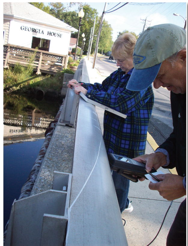
Figure 2.1. Volunteers monitor water quality off of a bridge in Laurel, Delaware, in a creek that drains into the Nanticoke River. Volunteers are a critical part of a monitoring program.
