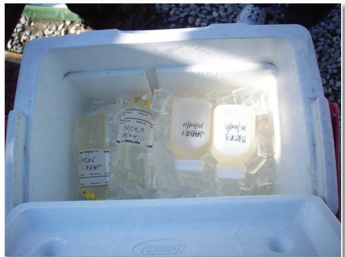
Figure 5.4. Labeled water samples are placed in a cooler with ice to preserve the integrity of the sample.
