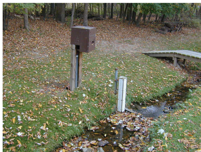
Figure 2.8. A stream gage can be installed by securing it to bedrock to record the height of the water.
