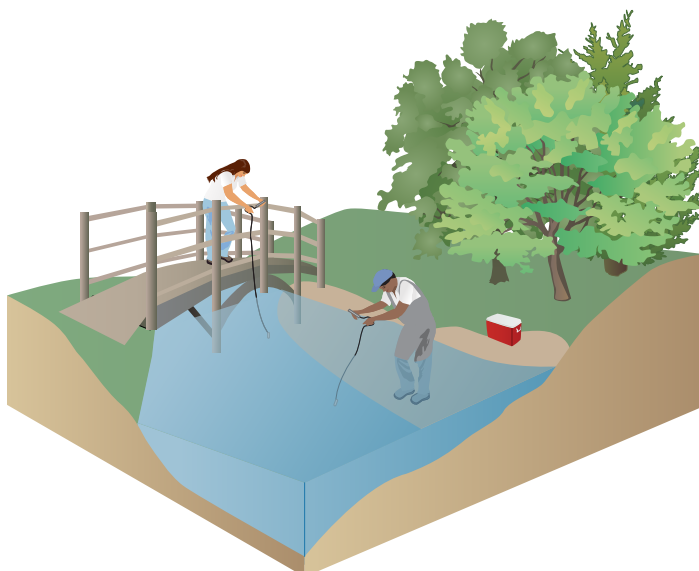
Figure 4.2. Sampling should be conducted from the middle of the stream, whether that is from a bridge or through wading.
