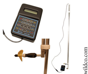
Figure 2.7. This photograph shows a streamflow meter that can be used to more accurately measure flow.
