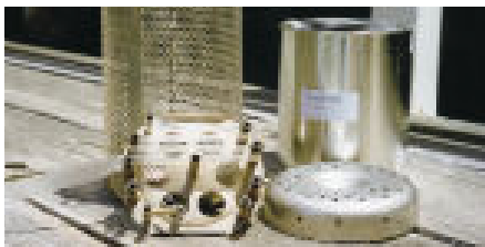
Passive sampling device (PESD) used to measure organic pollutants in water.
