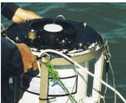
Spectroradiometer used to measure spectral properties of the water
