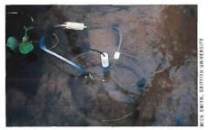
Dissolved oxygen probe inserted in transparent plastic dome to measure GPP and Rat of a cobble on the stream bed.
