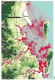
Mesh of the Moreton Bay Receiving Water Quality Model, showing the representation of the Bay as a network of onedimensional and two-dimensional elements, with a spatial resolution ranging from 330 m – 2000 m. The model includes hydrodynamic, transport and water quality components.
