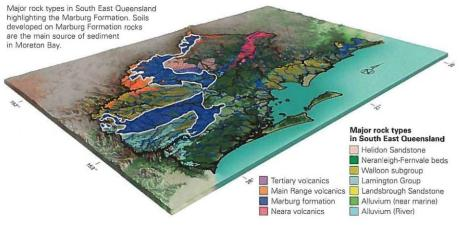
The modelling predicts that about 70% of the sediment is generated from subcatchments that occupy less than 30% of the region as a whole. This outcome is consistent with spatial tracing results, which show that most of the sediment produced in the Brisbane and Logan catchments originates from soils developed on Marburg Formation rocks.
