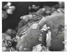
Scanning Electron Microscope image of suspended solids collected from Jindalee 22/11/00.
