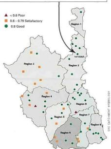
Estimates of flow in EMSS were calibrated against data from gauging stations in SEQ.
