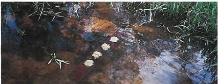
Algae bioassay technique: Wooden tray with four small, plastic pots filled with 4 different nutrient treatments (no nutrients, N, P, and N + P) and covered with fine mesh were deployed in-stream. After 21 days, the trays were collected, the mesh removed and chlorophyll a concentrations (algal biomass) measured.
