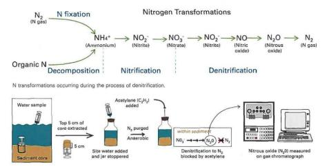
Denitrification methodology using acetylene blockage technique.
