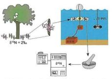
Methodology for tracing Sewage: The macroalgae Catenella nipae, is collected on mangrove pneumatophores and deployed in clear chambers at half secchi depth, and exposed to ambient water for four days. Samples are then collected, dried and analysed for 8<sup>th</sup> Value on a mass spectrometer.
