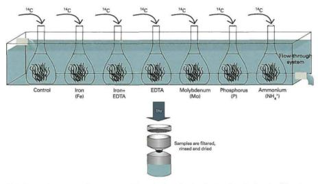
Methodology used to assess the effects of nutrient additions on Lyngbya majuscula productivity using radioactive Carbon (14C) uptakes.
