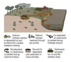
Erosion processes were traced using the isotopes cesium (<sup>137</sup>Cs) and radium (<sup>228</sup>Ra). Used in combination, these two radionuclides can give a good indication about where sediment has originated from in the landscape.
