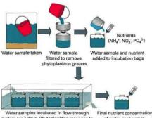
system for 7 days. Phytoplankton response to nutrient addition is monitored using florometry determine phytoplankton (see O'Donohue et al 1998)
