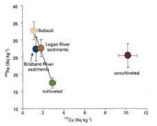
Average radium (<sup>288</sup>Ra) and cesium (<sup>137</sup>Cs) values from cultivated and uncultivated soils (hillslope erosion) and subsoils (channel erosion), compared with average values obtained from sediment in the lower Brisbane and Logan Rivers. These results show that the river sediments mainly originate from subsoil erosion (75%), with most of the remaining sediment coming from erosion of cultivated soil.
