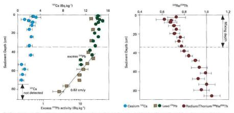
Sediment core profiles of isotopes used to determine sedimentation rates in Moreton Bay. Active mixing of the upper 35 cm of sediments occurs after sediment is deposited. Below this depth, sediment accumulation rates can be measured.
