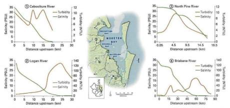
Turbidity and salinity longitudinal profiles of four Moreton Bay river estuaries. The physical processes in the turbid Brisbane and Logan Rivers appear similar as the position of the turbidity maxima corresponds to the intrusion of salinity.
