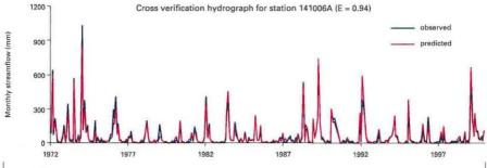
For the EMSS to yield reliable estimates of pollutant loads, it is essential that the flow predictions from the model are accurate. Getting this right was a two-step process.
