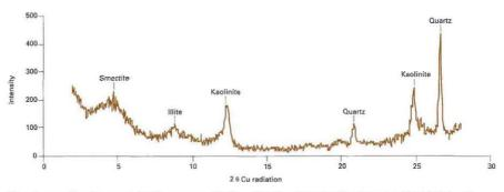
Mineral composition of suspended solids as measured by X-ray diffraction of the clay mineral structure. The labelled peaks correspond to a known diffraction pattern of each clay mineral structure.
