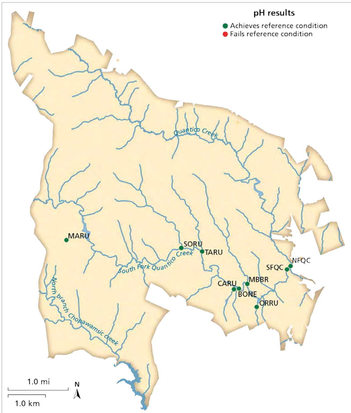
Figure 4-25 Attainment of pH reference condition by site from 2005 to 2013 for 9 stream sampling locations near PRWI. Site medians were used for this analysis.
