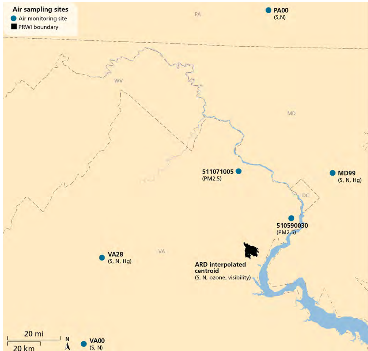
Figure 4-61 Regional air quality monitoring sites for wet deposition of sulfur and nitrogen, ozone, visibility, particulate matter, and mercury deposition. Wet deposition, ozone, and visibility data for 2006-2010 were interpolated by NPS ARD to estimate mean concentrations for PRWI.
