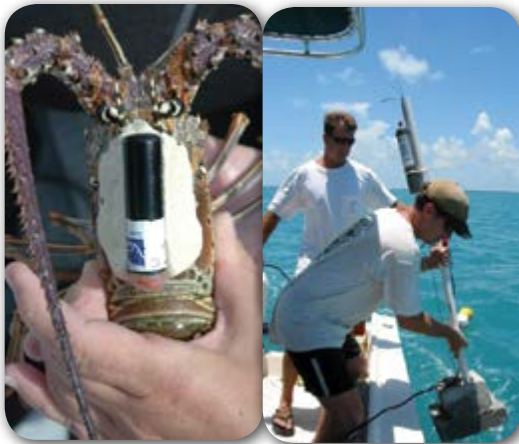
Left: Lobsters can be tracked using miniature acoustic tags that ping their location to acoustic receivers. Right: Scientists deploy an acoustic receiver to track spiny lobster movement.
