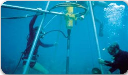
Scientists use a pneumatic coring device to obtain coral cores.
