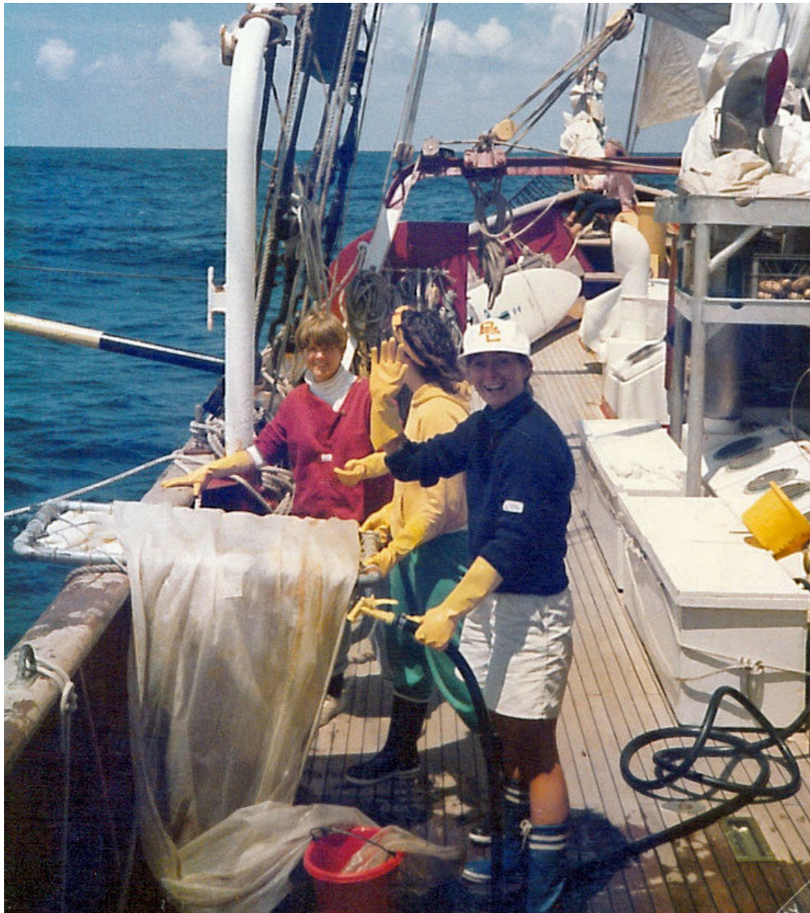
Retrieving a surface plankton net aboard R/V Westward as part of Sea Semester.
