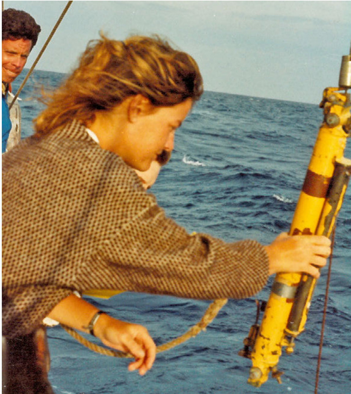
Collecting water samples using Nansen bottles aboard R/V Westward.
