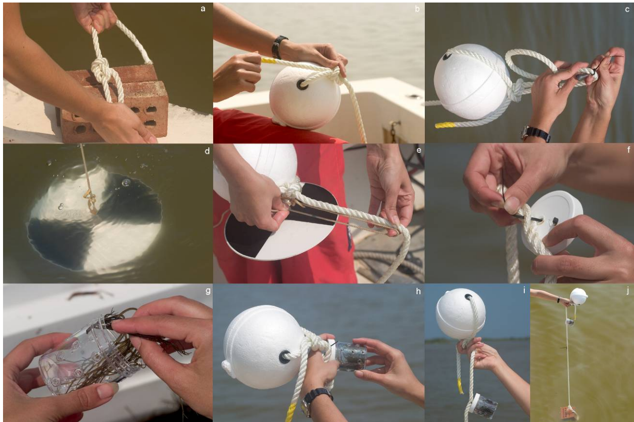
Plate 1. Preparation of the macroalgal \delta^{15}\text{N} incubation rig: a) securing rope to bricks for anchor; b) tying on the buoy; c) zip tying a sinker part way down the rope to keep the chamber under water; d) measuring the Secchi depth; e) finding the point on the rope that is half the Secchi to standardize the light regime between sites; f) zip tying the chamber lid to the rope at ‘half Secchi depth’; g) placing approximately 5 g (wet wt) of macroalgae into the perforated chamber; h) screwing the chamber into its lid; i & j) deploying chamber at GIS located site.
