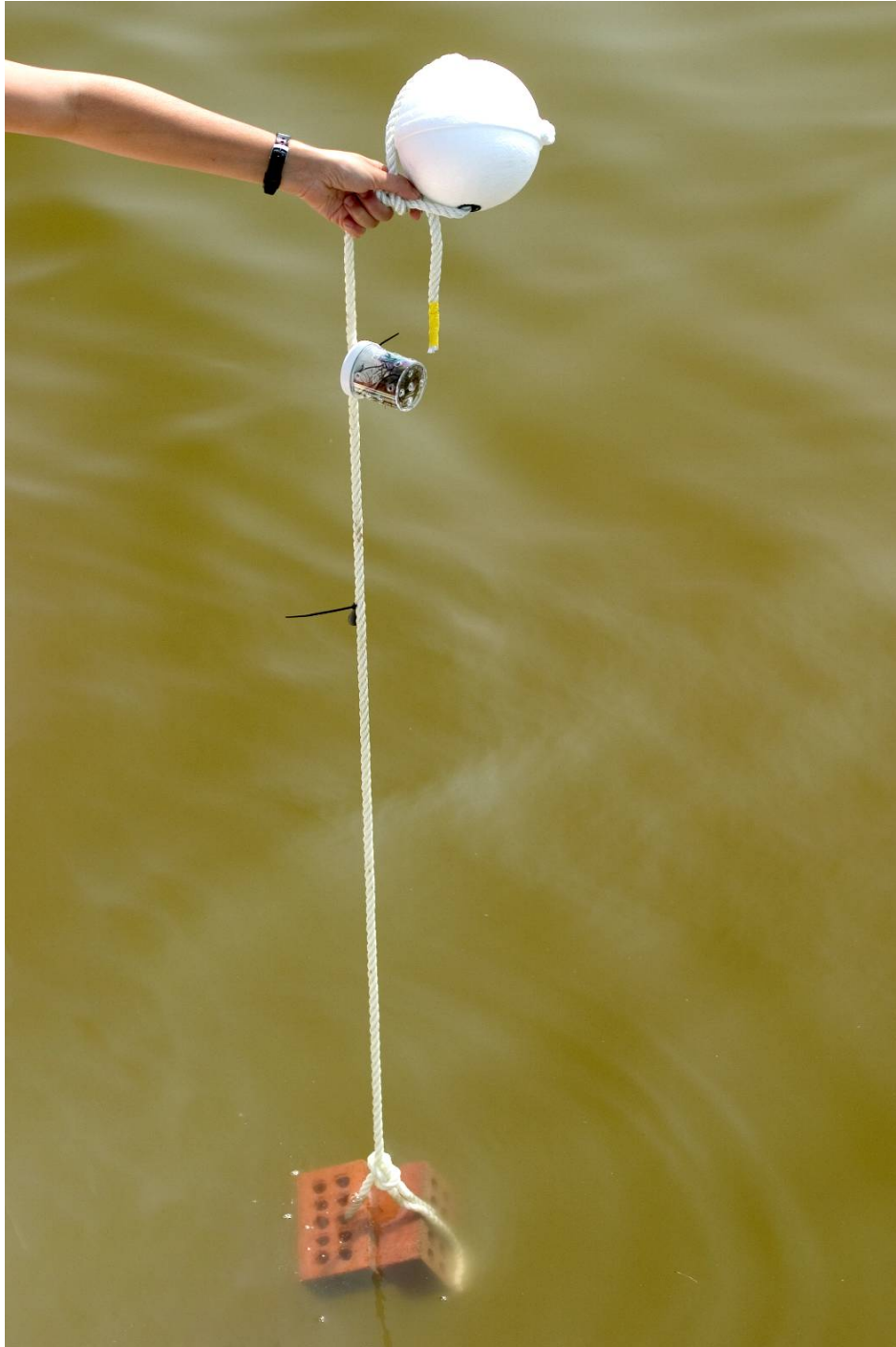
Plate 2. Close up of the macroalgal \delta^{15}\text{N} incubation rig with buoy, perforated macroalgal chamber, sinker and bricks.
