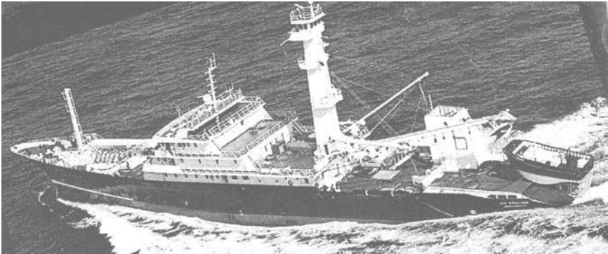
Fig. 7. A modern tuna clipper. A pad just after the mast is for a helicopter used to spot schools of tuna. Source: Fisheries News International.
