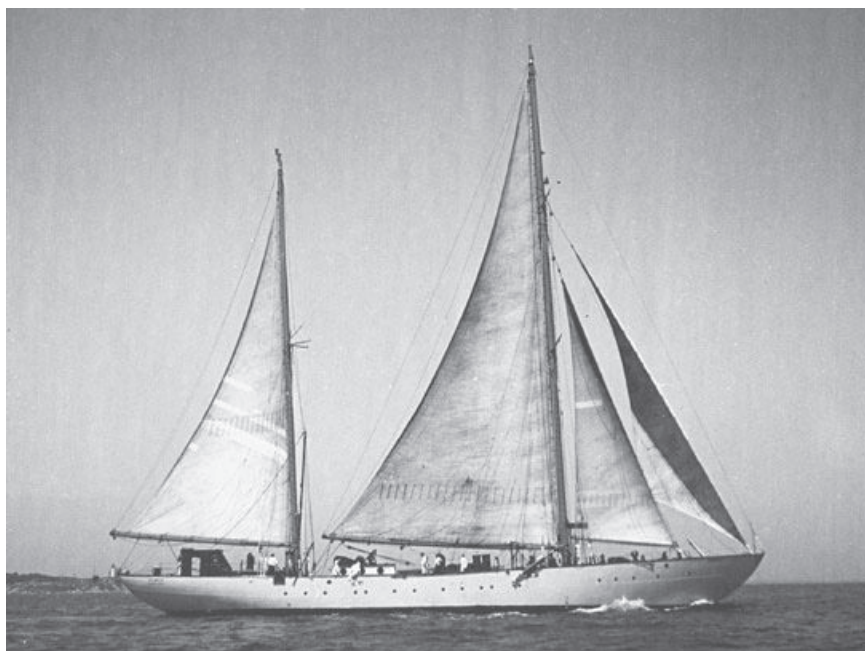
Fig. 4. R.V. Atlantis on a close reach. Atlantis was the first high seas research vessel of the Woods Hole Oceanographic Institution. Launched in Denmark in 1932, she was a 149 foot steel hulled ketch with a powerful auxiliary engine. Courtesy of the Woods Hole Oceanographic Institution.
