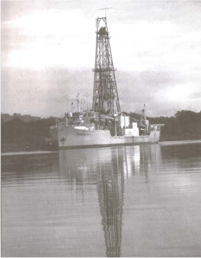
Fig. 4. Joides Resolution of the Ocean Drilling Program passing through the Panama Canal. This ship deployed 9,200 m (30,000 feet) of drill string and used computer-controlled positioning regulated by 12 thrusters. Joides Resolution is being modernized and will complement the work of a behemoth drill ship built in Japan. Source: The original Ocean Drilling Program.
