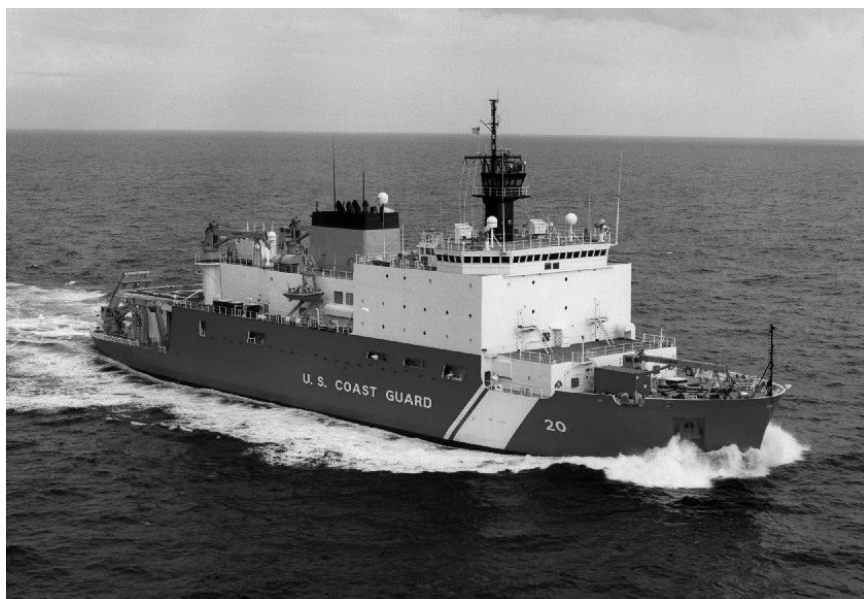
Fig. 20. USCG Healy. This is the largest of the icebreakers, having been built to serve both as an ice breaker and as an Arctic oceanographic research ship. The hull color is solid red which is customary for ice breakers of the U.S. Coast Guard fleet. Source: NOAA.
