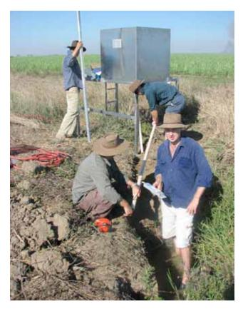
Figure 13.1 – Automated sampler in the Burdekin (Image: Zoe Bainbridge, Australian Centre for Tropical Freshwater Research).
