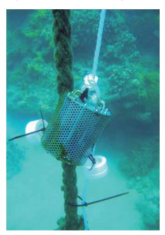
Figure 4.3 – Passive samplers monitor marine water pesticide concentrations (Image: J. Muller, University of Queensland).
