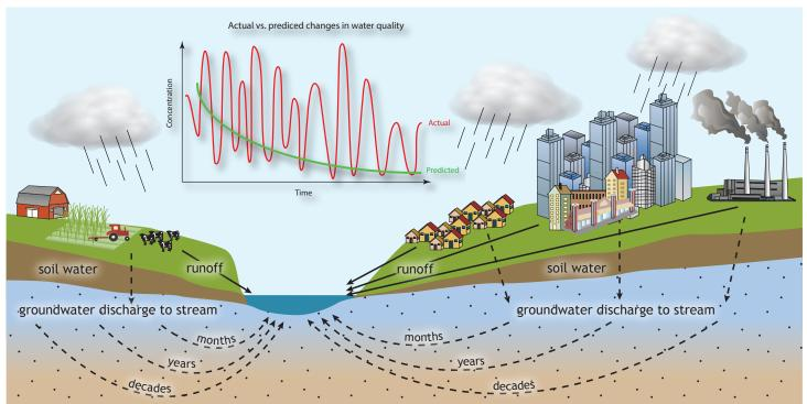
Conceptual diagram of the water cycle and major sources of nitrogen, phosphorus, and sediment pollution to Chesapeake Bay. Once in groundwater, nitrogen can take from months to years to be transported to rivers and the estuary which, combined with variable water quality and precipitation, can make detecting improvements difficult.
