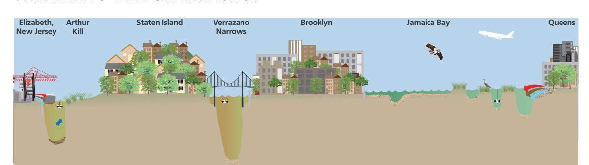
Arthur Kill, separating New Jersey from Staten Island, is maintained as a dredged shipping channel (35' deep) with Harbor with vigorous tidal poor flushing.
