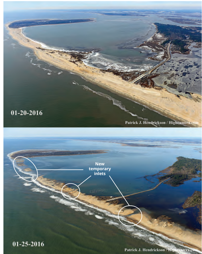
The top photo shows an intact southern end of Assateague Island prior to the blizzard of 22–24 January 2016. That storm breached Assateague Island in several places, as seen in the bottom photo. Photos by Patrick J. Hendrickson/Highcamera.com
