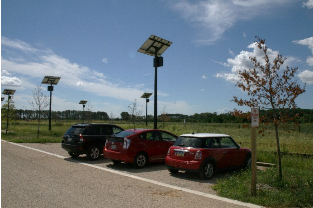
Impervious surfaces like this parking lot at the Harriet Tubman Underground Railroad National Historical Park visitor center limit the filtering of runoff by soil, resulting in increased levels of nutrients entering waterways. Photo: Todd Lookingbill, September 2016.
