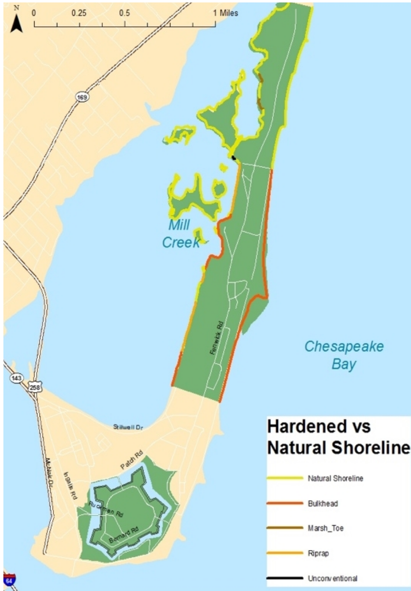
Figure 4-25. Natural vs hardened shoreline in Fort Monroe National Monument (Data source: VIMS 2011).
