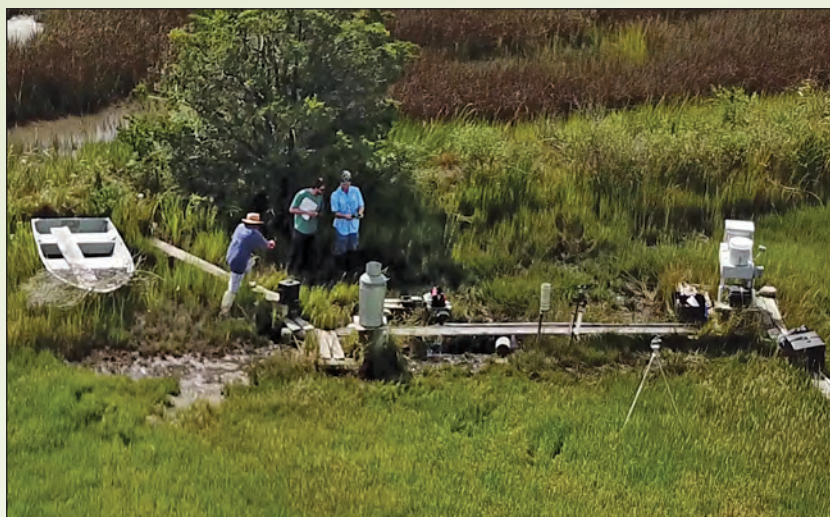
Figure 5.S1. A network of atmospheric deposition sampling combined with precipitation measurements provides estimates of nitrogen loads to the Chesapeake Bay watershed. Photograph by Environmental Engineering and Measurement Services, Inc., used with permission.
