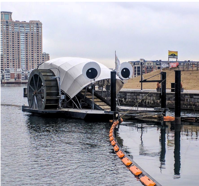
Mr. Trash Wheel (introduced in 2014) in the Baltimore Harbor. The orange buoys help direct floating trash into his mouth. Professor Trash Wheel (2016), Captain Trash Wheel (2018), and Gwynnda the Good Wheel of the West (2021) are his 3 siblings also found in the harbor.
