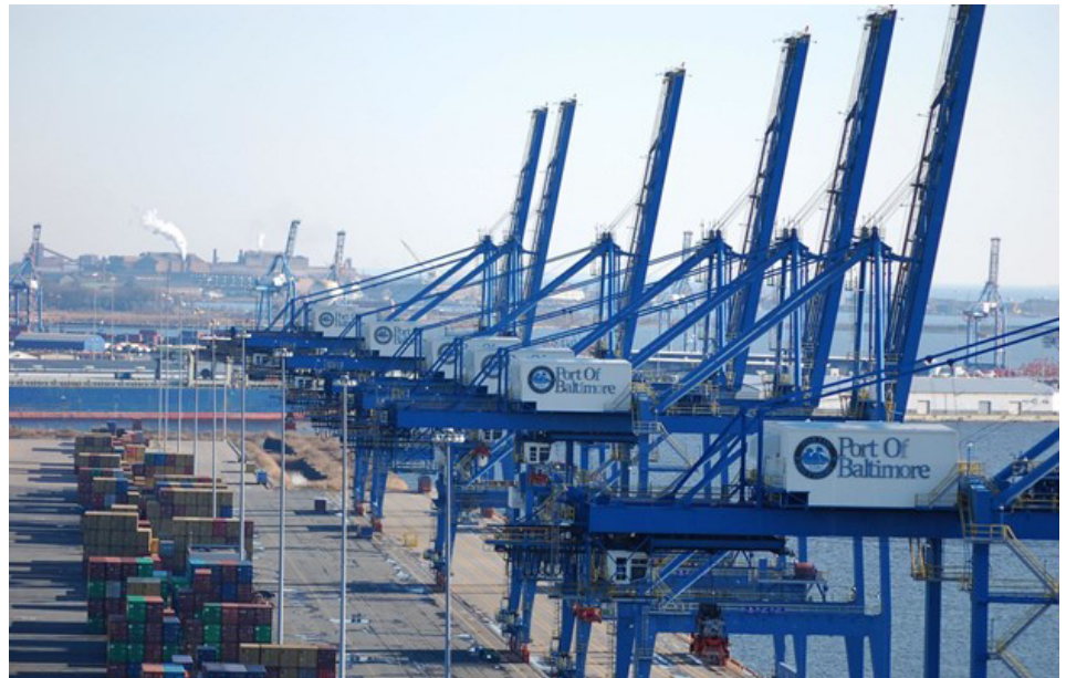
A row of port cranes lining the Baltimore Harbor. These cranes load large shipping containers from ships to land.
