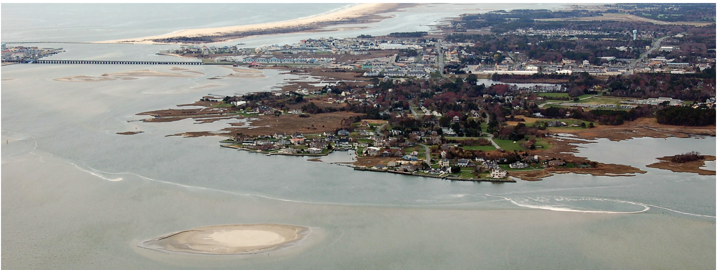
This photo shows Tern Island in Isle of Wight Bay in the foreground, one of four islands constructed in the Coastal Bays in 2013/14 to provide new habitat for colonial nesting birds. All four islands have since disappeared due to erosion and changes in currents. Photo by Kathy Phillips.
