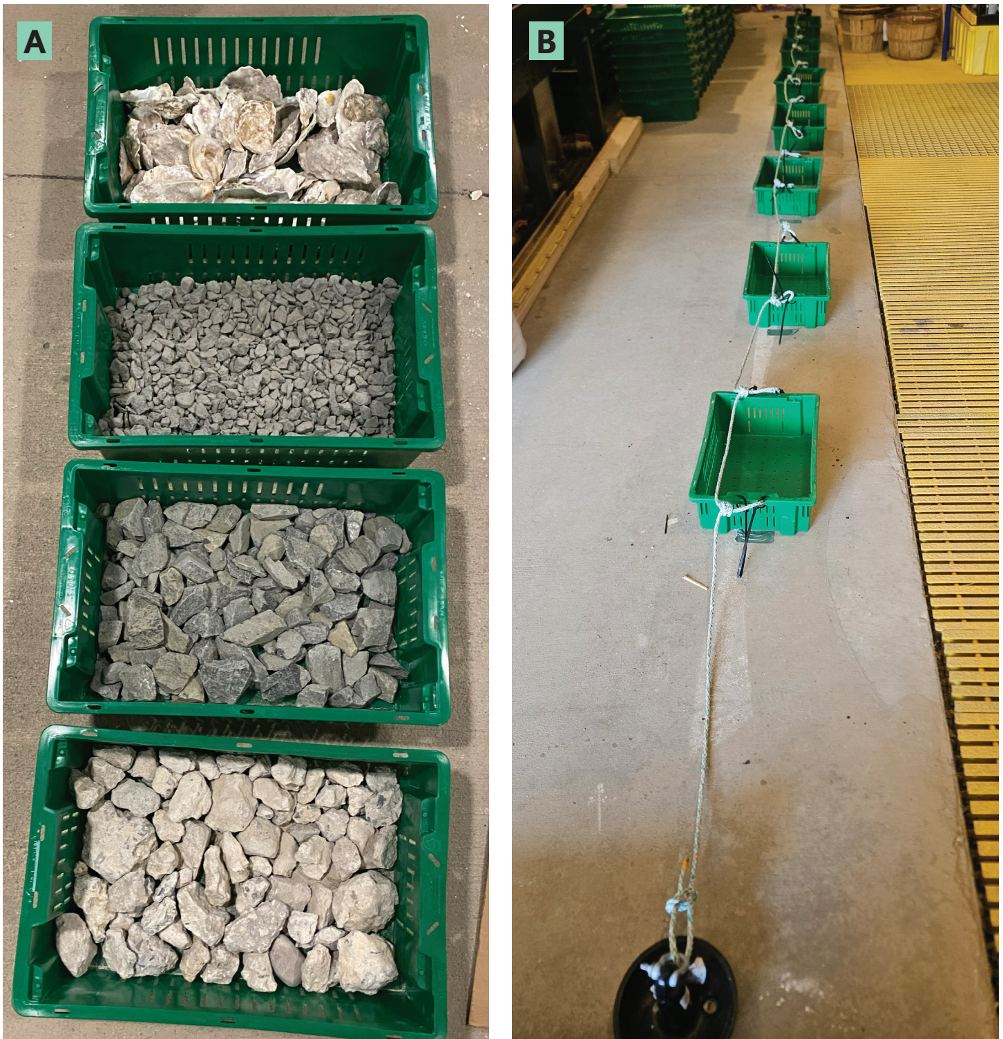
Figure 1B.2 Example of alternative substrates and lines of trays before deployment. A) Trays with alternative substrates (bottom to top: clean crushed concrete, Havre de Grace stone, granite, and fresh Eastern oyster shell). B) Fully assembled line of trays. Lines had seven trays with each type of material in randomized order. Four or five lines of trays were deployed at each site. Photos by Elizabeth North.
