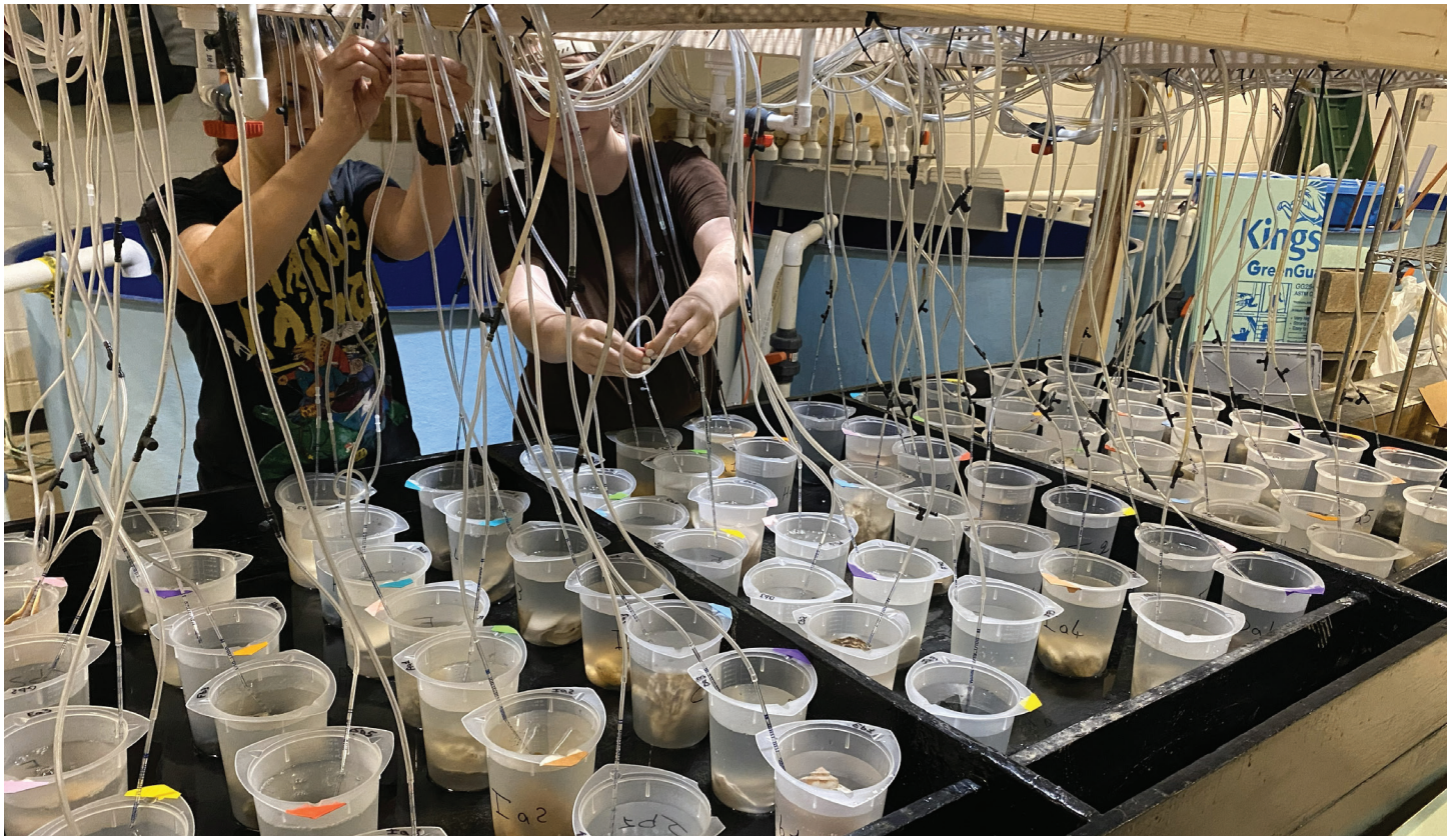
Figure 1A.2 Experimental setup on a flow-through table that delivered Choptank River water to each of the 80 containers that were equipped with individual air lines. The same number of Eastern Oyster larvae were introduced to 50 of the containers on June 10, 2024. The remaining 30 containers were sampled periodically for water quality and metals leaching. Monica Fabra and Evan Merk are pictured setting up the system. Photo by Elizabeth North.
