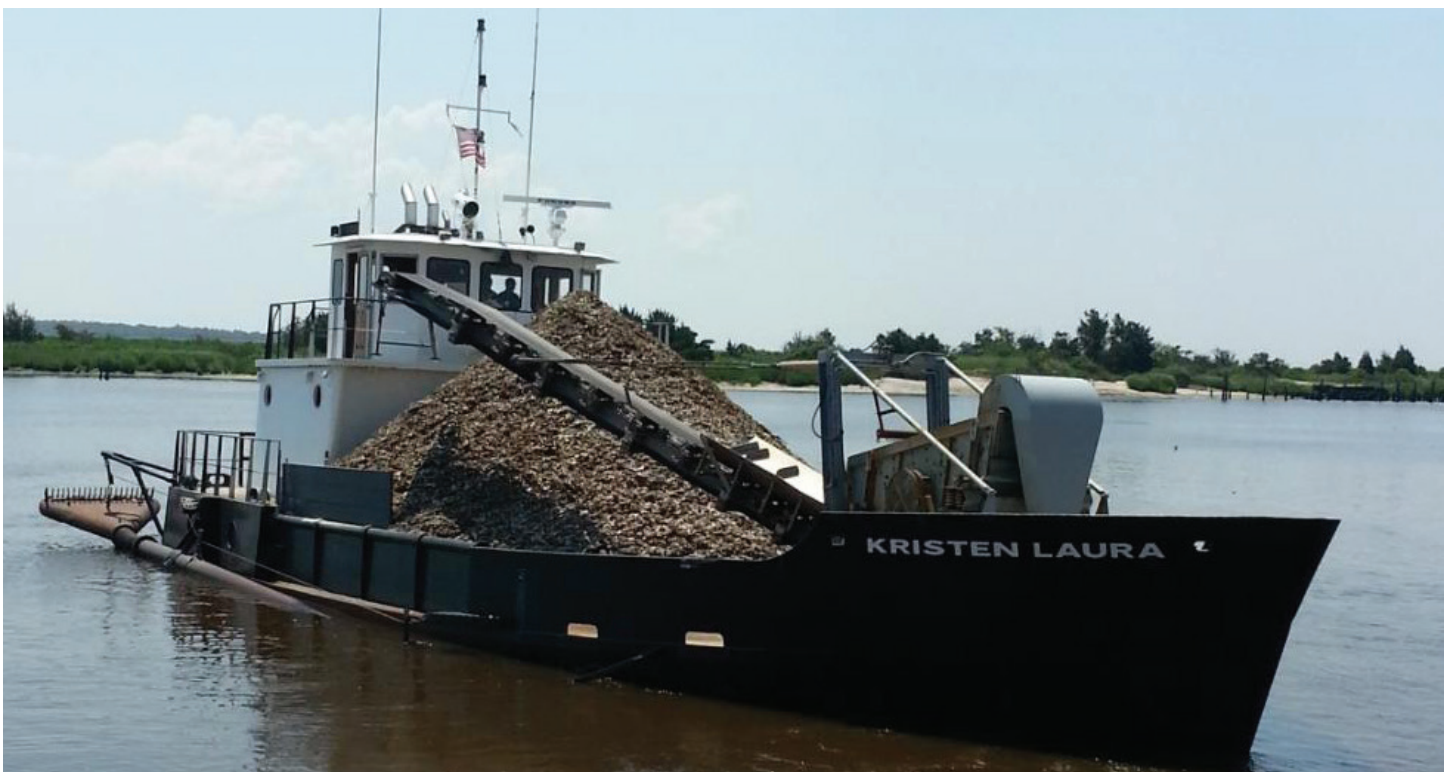
Figure 3.4 Suction dredge boat with a load of dredged shell in Delaware Bay. The head of the suction dredge is at the stern. Photo courtesy of Steve Fleetwood.
