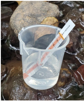
Hach chloride testing strip used by LWC volunteers.
