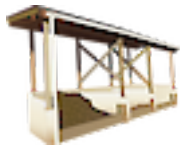
Manure composting bunker
